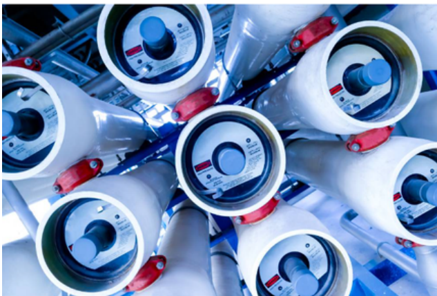
Nano Filtration Unit
