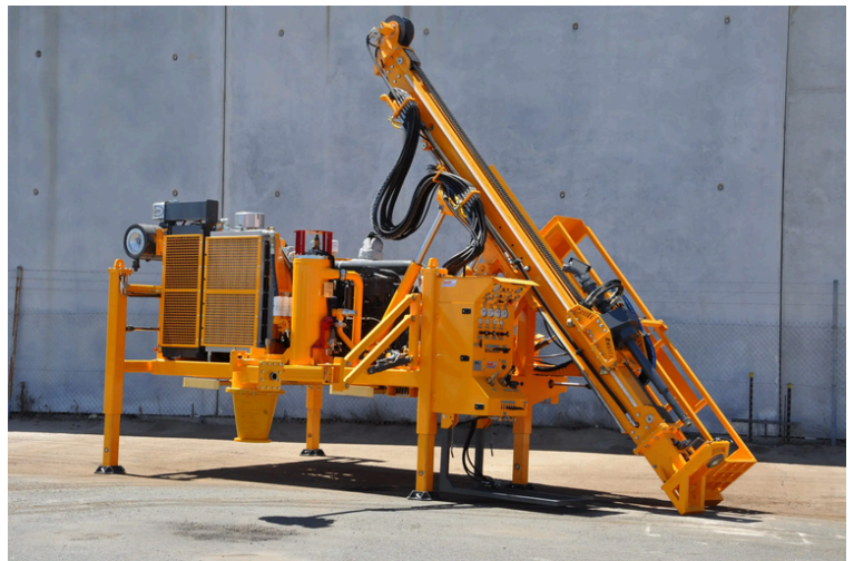
Air Core Drill Rig
