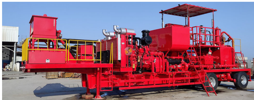
Twin Pump Cementing Unit
