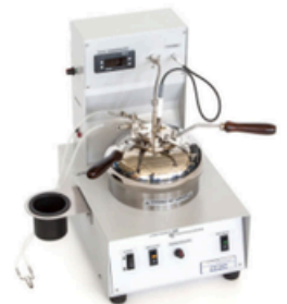
Flash point by Tag Closed Tester
