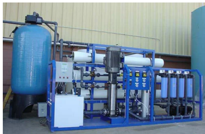
Reverse Osmosis System
