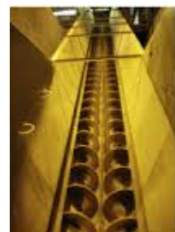
Screw Conveyor System
