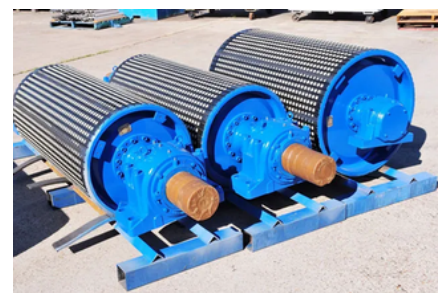
Conveyor Drive Pulley
