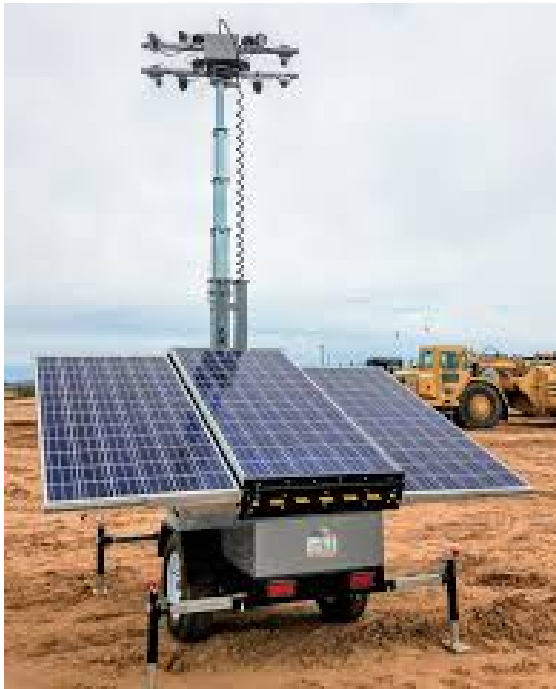
Solar Lighting set
